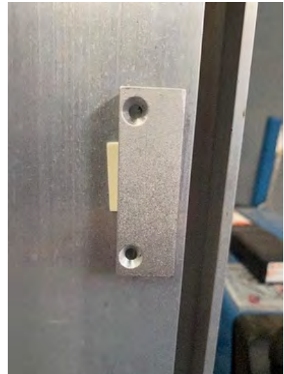
Figure 11. Magnetic component attached to the backbone
