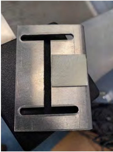
Figure 12. Two-sided tape on the bracket
