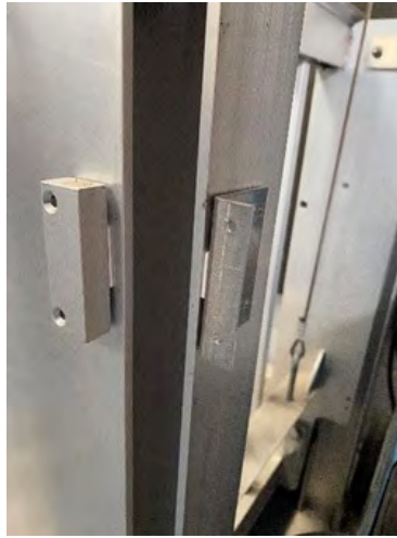
Figure 13. Bracket tapped to the back of the travel beam
