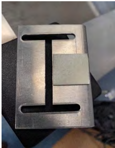
Figure 12. Two-sided tape on the bracket
